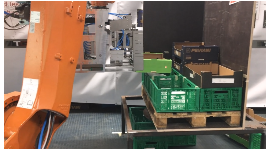
Fig. 1: Experimental setup: robot with custom end-effector for palletizing cartons. See [7] for a video of the experiments.
